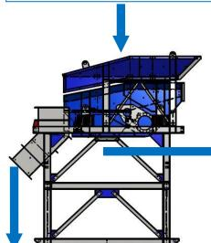
2) Oversize Rocks are discharged while undersize material (-150mm / -6") falls into the CS-120 Trommel Feed Chute 3) The CS-120 Trommel thoroughly scrubs all material in the 3-chamber high-retention-time Scrubber. Material is then split into undersize and oversize fractions in the screening section (\*)
